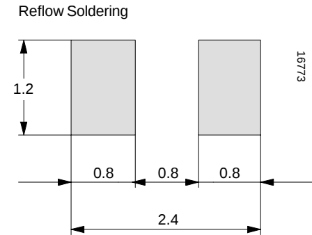
Figure 2. Recommended foot pads (in mm)
