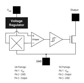
**Note:** Static sensitive device; please observe ESD precautions. Reverse  $V_{DD}$  protection is not included. For reverse voltage protection, a 100 **W** resistor in series with  $V_{DD}$  is recommended.
