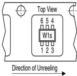
Marking on SOT-363 package (for example W1s) corresponds to pin 1 of device
