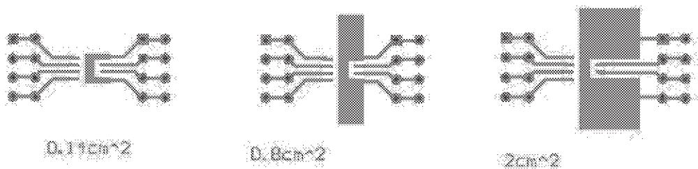
Layout condition of  $R_{th}$  and  $Z_{th}$  measurements (PCB FR4 area= 58mm x 58mm, PCB thickness=2mm, Cu thickness=35 $\mu$ m, Copper areas: 0.14cm<sup>2</sup>, 0.8cm<sup>2</sup>, 2cm<sup>2</sup>).
