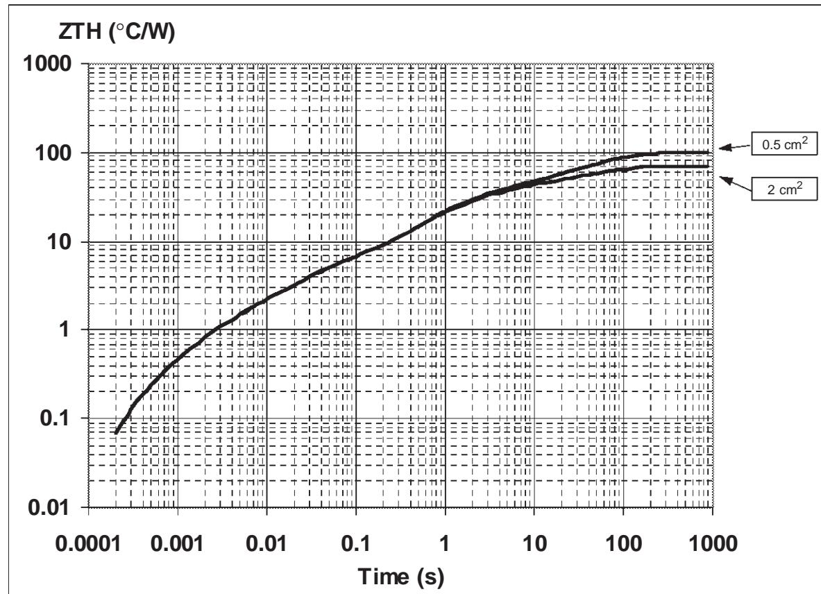
Thermal fitting model of a single channel HSD
