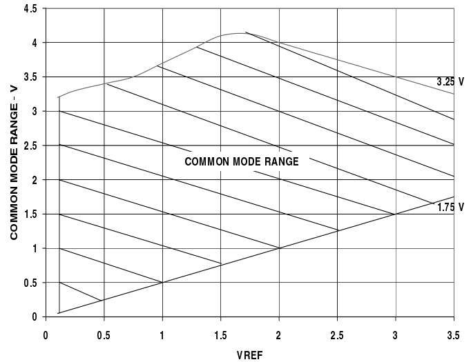
Figure 9. Input Common Mode Range versus V_{REF} ( V_{DD} = 5V and V_{REF} (max) = 3.5V )
