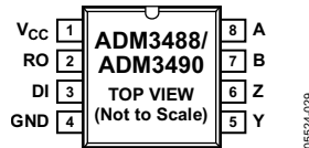
Figure 5. ADM3488/ADM3490 Pin Configuration
