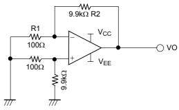
$$SVR(-) = 20log \left| \frac{\Delta V_{EE} \times 100}{\Delta VO} \right|$$
