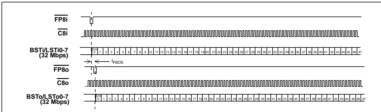
Figure 7 - Input and Output (Generated) Frame Pulse Alignment
