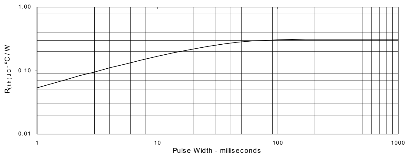
Fig. 13. Maximum Transient Thermal Resistance
