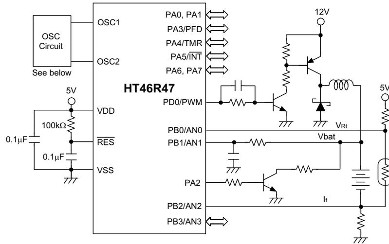
Note: The resistance and capacitance for reset circuit should be designed to ensure that the VDD is stable and remains in a valid range of the operating voltage before bringing RES to high.
