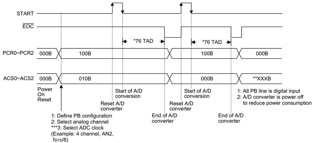
Note: \*\*\*\*\* A/D converting time is 76 TAD
