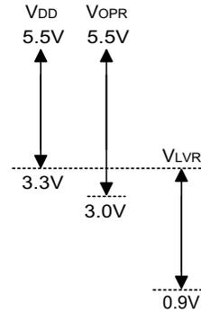
Note:  $V_{OPR}$  is the voltage range for proper chip operation at 4MHz system clock.
