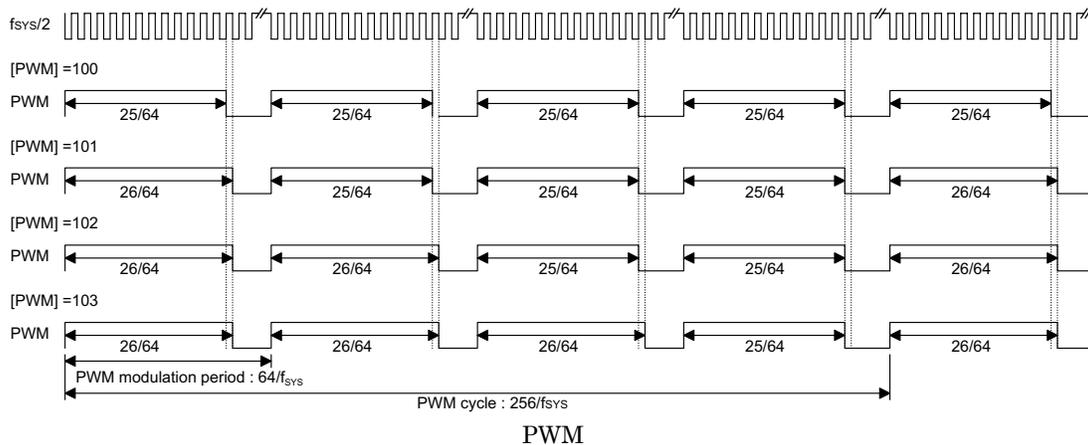
In a PWM cycle, the duty cycle of each modulation cycle is shown in the table.
