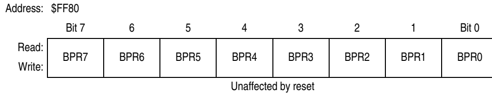
Figure 2-4. FLASH-1 Block Protect Register (FL1BPR)
