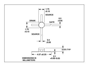
base station receiver in PCS, Japanese PHS, AMPS, GSM and other communications systems. The CFB0301 is in an industry-standard 70 mil package. It is surface mountable and available in tape and reel.
