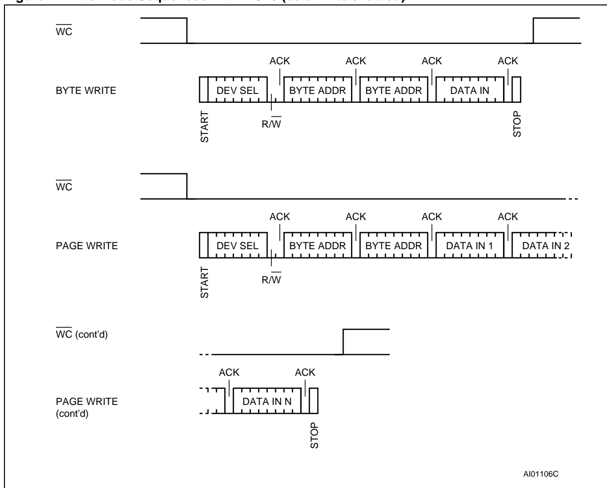
Figure 7. Write Mode Sequences with WC=0 (data write enabled)
