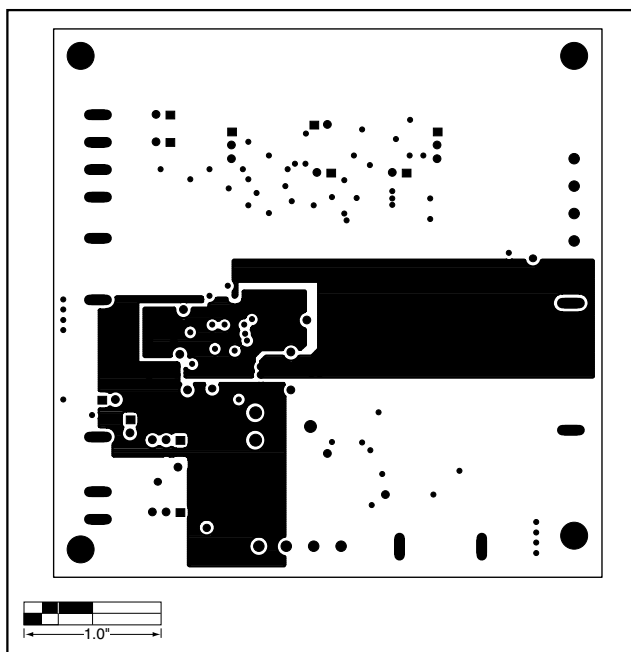
Figure 8. MAX1773 EV Kit PC Board Layout—Inner Layer 3
