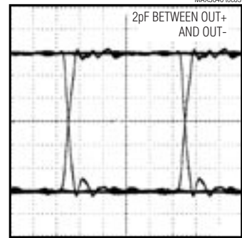
ELECTRICAL EYE DIAGRAM ( I_{MOD} = 30mA , 622.08MHz, 2^7 - 1 PRBS)
