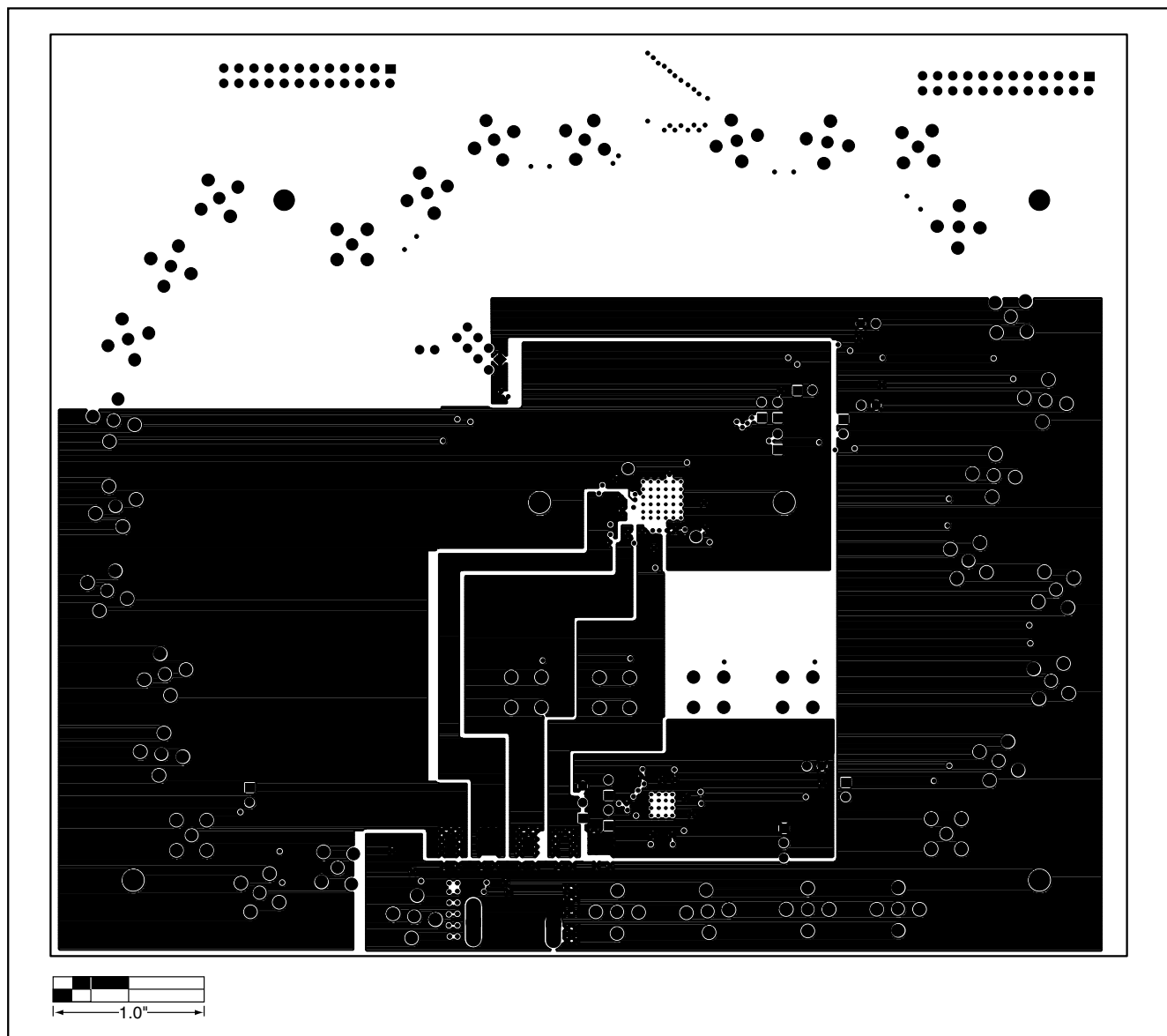
Figure 6. MAX3831/MAX3832 EV Kits PC Board Layout—Power Plane
