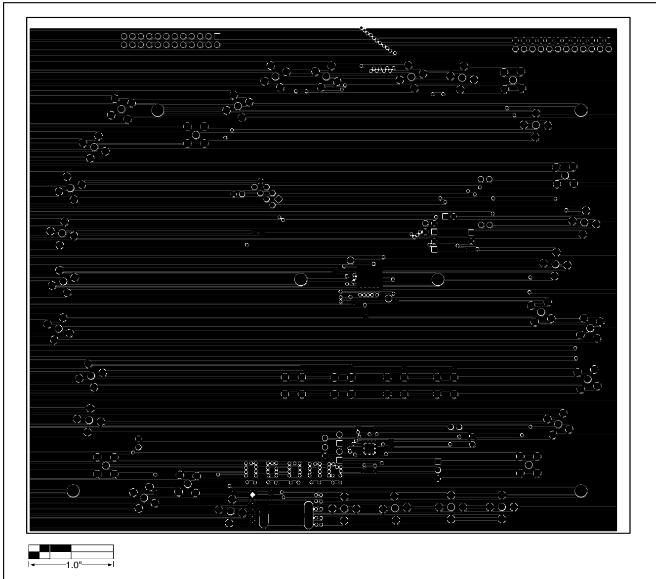
Figure 7. MAX3831/MAX3832 EV Kits PC Board Layout—Ground Plane
