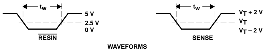
Figure 2. Input Pulse Definition
