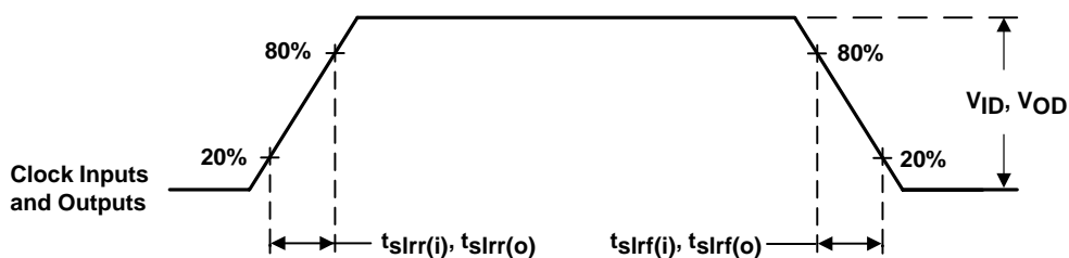
Figure 8. Input and Output Slew Rates
