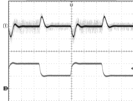
1.28MHz, 8.5V Application Boost Load Step
