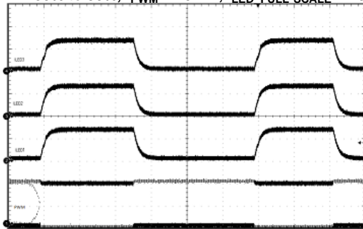
Ch1 = 2V/div; Ch2-4 = 10 mA/div; 2 msec/div
