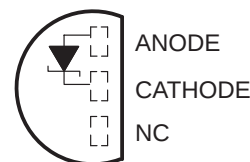
1.2 V . . . LP (TO-92/TO-226) PACKAGE (TOP VIEW)
