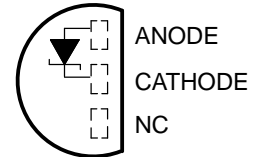
1.2 V . . . LP (TO-92/TO-226) PACKAGE (TOP VIEW)
