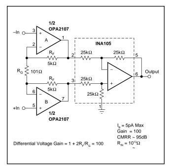
FIGURE 2. FET Input Instrumentation Amplifier.
