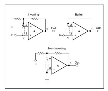
FIGURE 1. Connection of Input Guard.
