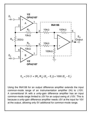
FIGURE 3. Precision Instrumentation Amplifier.
