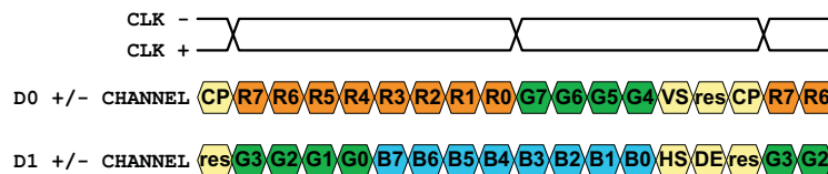
Figure 4. Data and Clock Input in 2-ChM (LS0 = high; LS1 = low)
