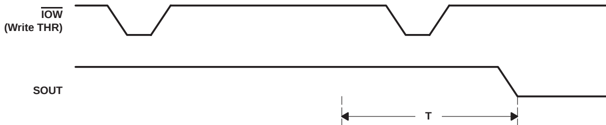
Figure 22. Error Case Timing Condition
