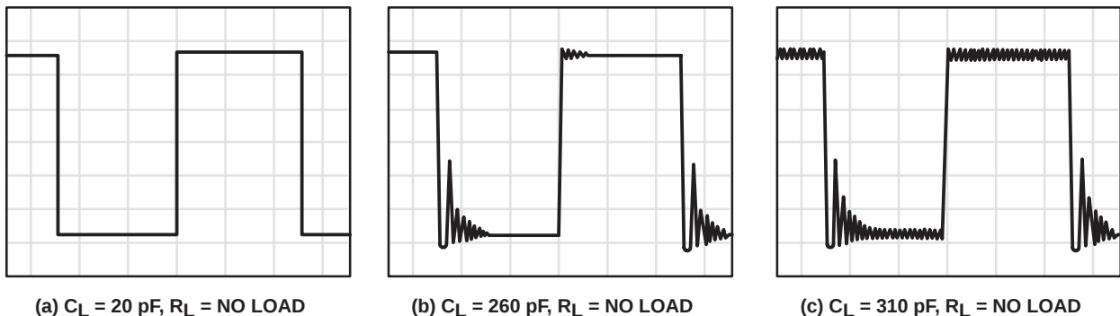
Figure 112. Effect of Capacitive Loads in Low-Bias Mode
