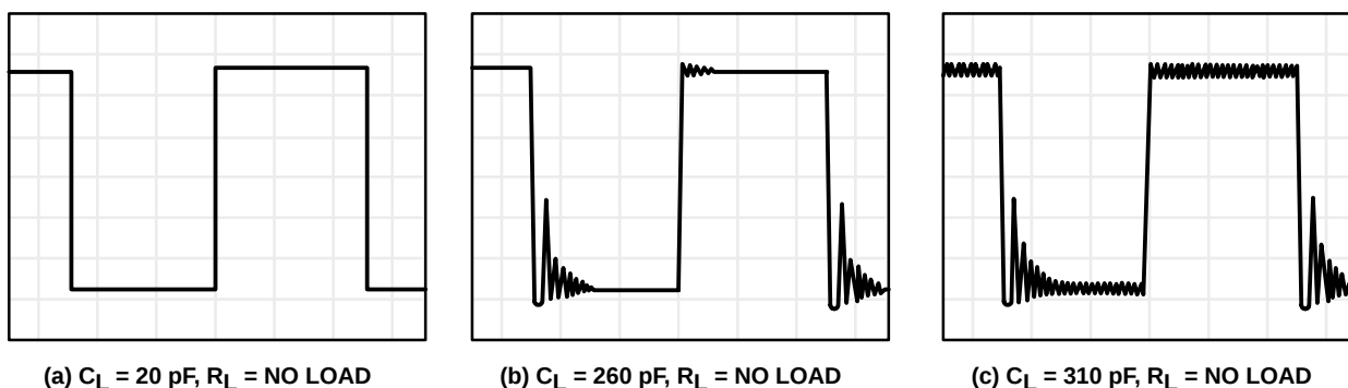
Figure 112. Effect of Capacitive Loads in Low-Bias Mode
