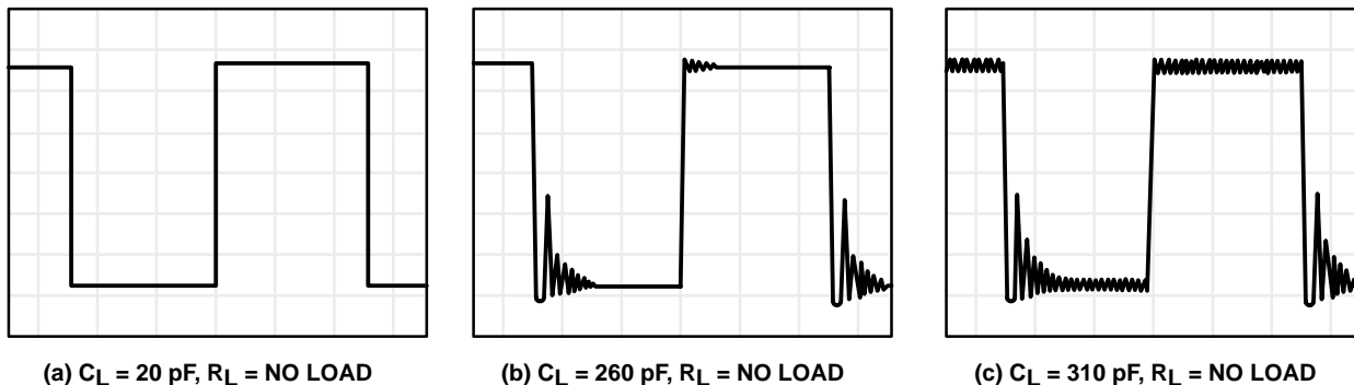
Figure 44. Effect of Capacitive Loads in Low-Bias Mode
