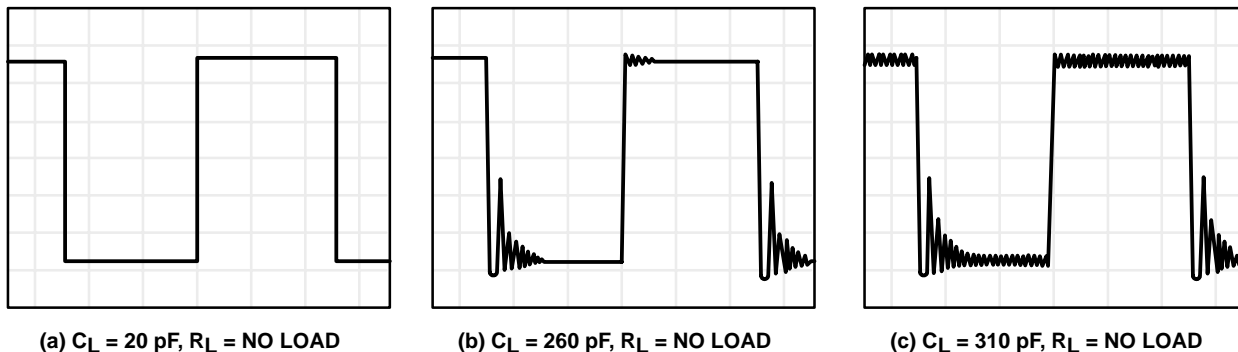
Figure 44. Effect of Capacitive Loads in Low-Bias Mode
