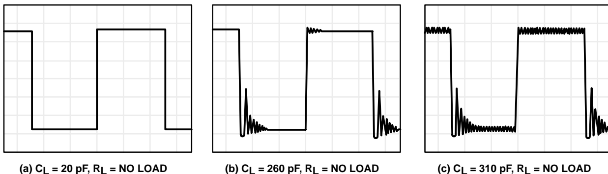
Figure 44. Effect of Capacitive Loads in Low-Bias Mode
