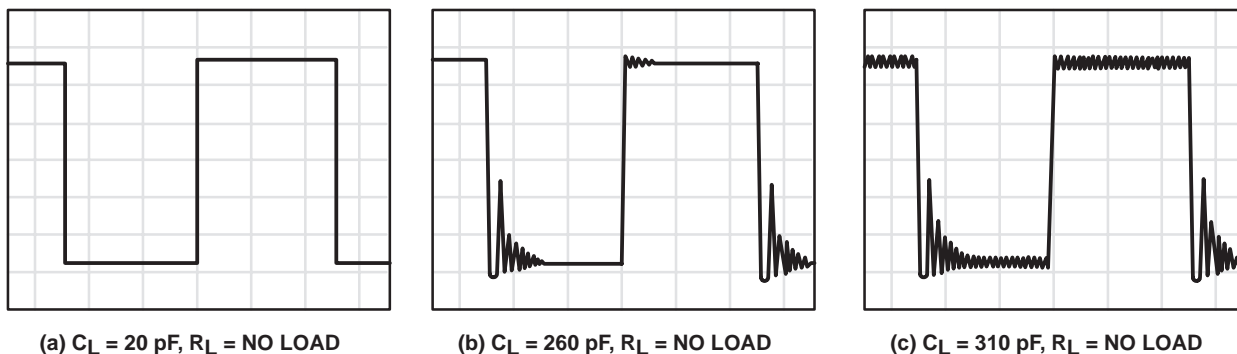
Figure 44. Effect of Capacitive Loads in Low-Bias Mode
