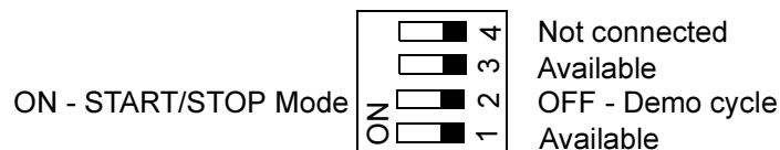
Figure 6. DIP Switch SW1
