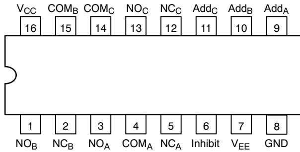
Figure 1. Pin Connection (Top View)
