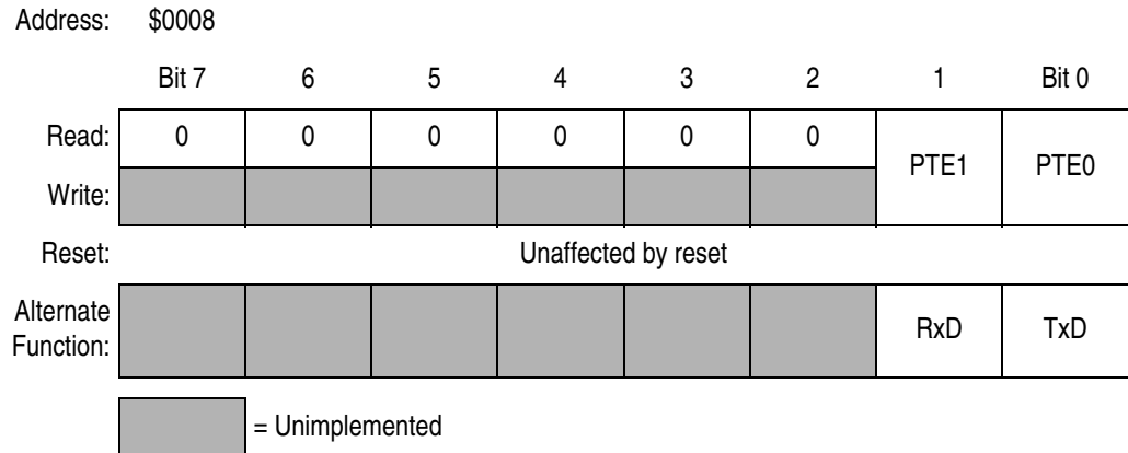
Figure 16-17. Port E Data Register (PTE)
