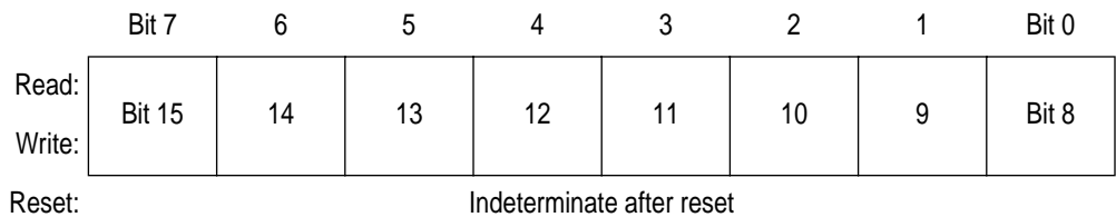
Figure 11-18. TIMA Channel 2 Register High (TACH2H)
