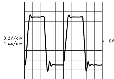
Large Signal Step Response V_S = \pm 1.35V, A_V = +1, Z_L = 10 k\Omega \parallel 20 pF, V_{IN} = 1 V_{PP}
