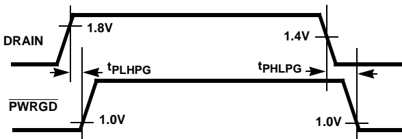
FIGURE 4A. DRAIN TO \overline{\text{PWRGD}} TIMING (ISL6140)
