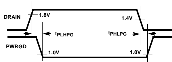
FIGURE 4B. DRAIN TO \overline{\text{PWRGD}} TIMING (ISL6150)
