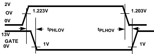
FIGURE 3A. OV TO GATE TIMING
