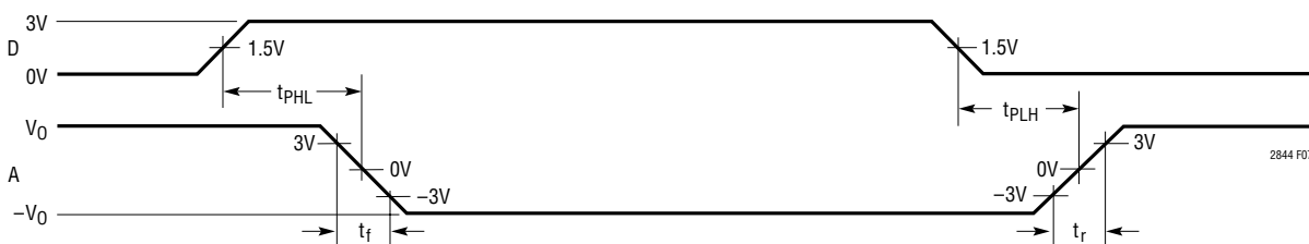
Figure 7. V.10, V.28 Driver Propagation Delays
