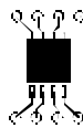
b) 105^\circ\text{C}/\text{W} when mounted on a .04\text{ in}^2 pad of 2 oz copper
