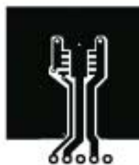
a) 40^\circ\text{C}/\text{W} when mounted on a 1\text{ in}^2 pad of 2 oz copper
