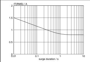
Fig.5. Maximum permissible repetitive rms on-state current I<sub>T(RMS)</sub>, versus surge duration, for sinusoidal currents, f = 50 Hz;  $T_{lead} \le 83$ °C.
