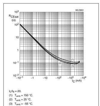
Fig.10 Equivalent on-resistance as a function of
