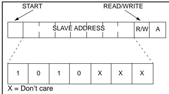
FIGURE 3-2: CONTROL BYTE ALLOCATION
