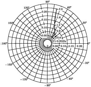
$S_{21e}$   $V_{CE} = 10V$   $I_{C} = 5mA$   $T_{a} = 25^{\circ}C$
