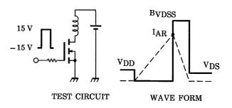
$$\begin{split} RG &= 25~\Omega \\ V_{DD} &= 25~V,~L = 471~\mu H \end{split} \qquad EAS = 0.$$
