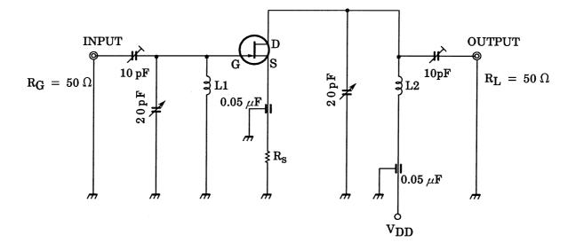
$L_1{:}~0.8~\text{mm}\phi~\text{A}_g$  plated Cu wire, 3 turns, 10 mm ID, 10 mm length.
