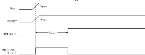
Figure 16. MCU Start-up, RESET Tied to V<sub>CC</sub>.
