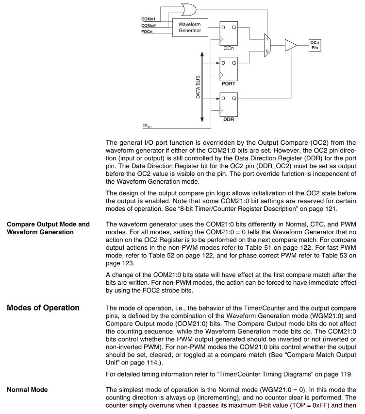
Figure 56. Compare Match Output Unit, Schematic
