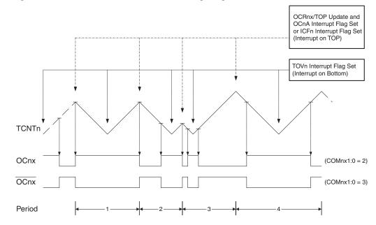
Figure 47. Phase Correct PWM Mode, Timing Diagram
