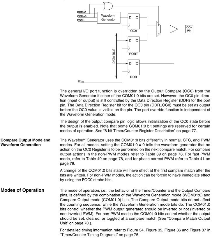
Figure 30. Compare Match Output Unit, Schematic
