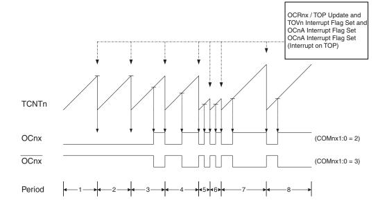
Figure 46. Fast PWM Mode, Timing Diagram
