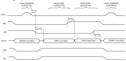
**Figure 135.** Parallel Programming Timing, Reading Sequence (within the Same Page) with Timing Requirements<sup>(1)</sup>
