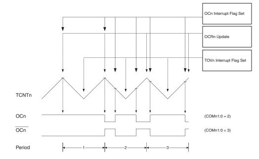
Figure 59. Phase Correct PWM Mode, Timing Diagram
