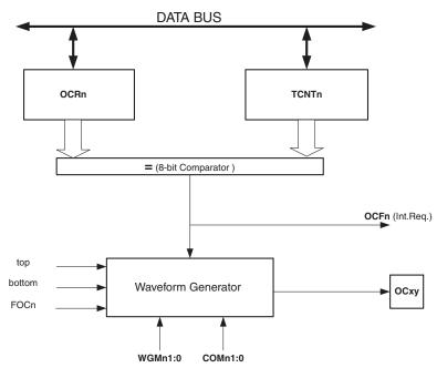
Figure 55. Output Compare Unit, Block Diagram
