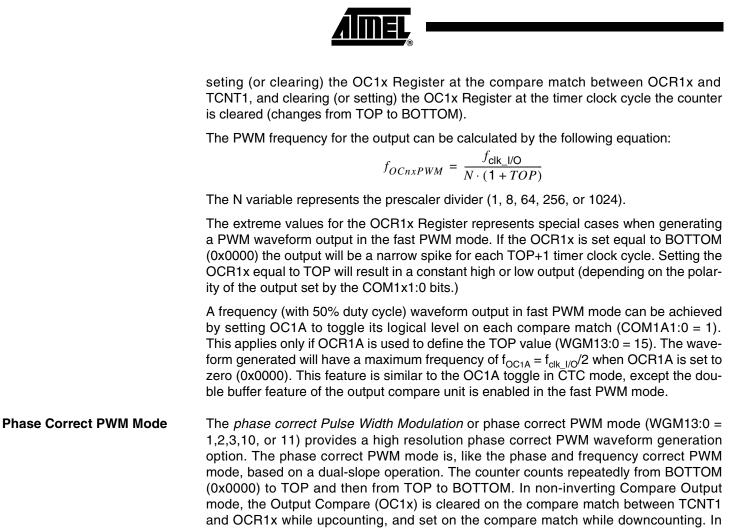
and OCR1x while upcounting, and set on the compare match while downcounting. In inverting Output Compare mode, the operation is inverted. The dual-slope operation has lower maximum operation frequency than single slope operation. However, due to the symmetric feature of the dual-slope PWM modes, these modes are preferred for motor control applications.
