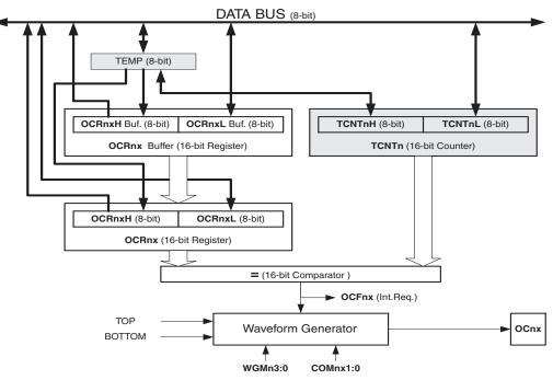
Figure 43. Output Compare Unit, Block Diagram
