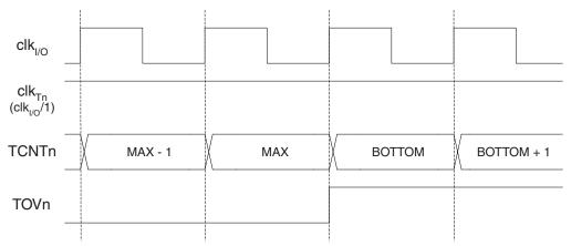
Figure 35 shows the same timing data, but with the prescaler enabled.
