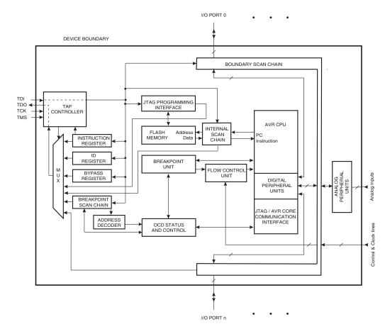
Figure 112. Block Diagram
