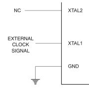
When this clock source is selected, start-up times are determined by the SUT fuses as shown in Table 12.
