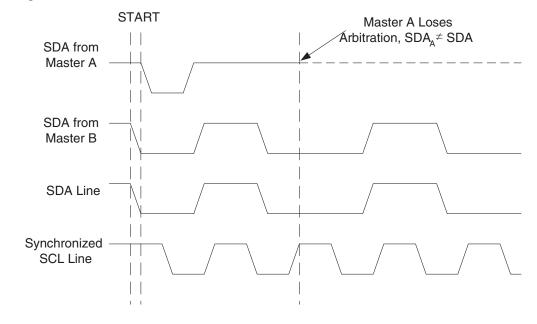
Figure 83. Arbitration between Two Masters
