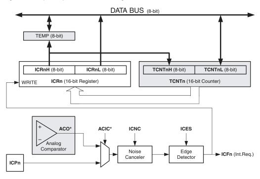
Figure 42. Input Capture Unit Block Diagram
