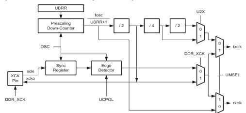
Figure 70. Clock Generation Logic, Block Diagram
