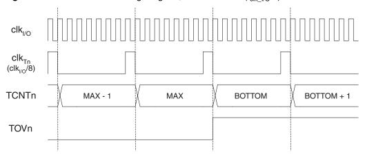
Figure 61. Timer/Counter Timing Diagram, with Prescaler ( $f_{clk\_l/O}/8$ )
