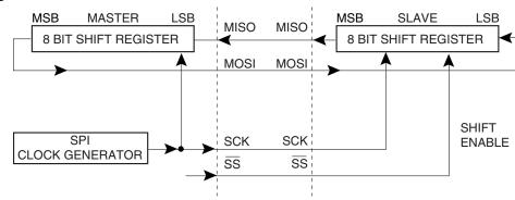
Figure 66. SPI Master-slave Interconnection
