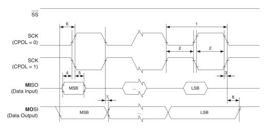
Figure 147. SPI Interface Timing Requirements (Slave Mode)
