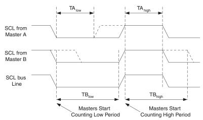
Figure 82. SCL Synchronization between Multiple Masters
