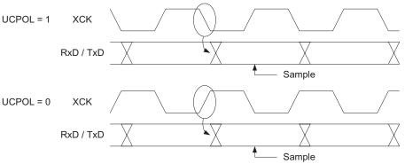
The UCPOL bit UCRSC selects which XCK clock edge is used for data sampling and which is used for data change. As Figure 71 shows, when UCPOL is zero the data will be changed at rising XCK edge and sampled at falling XCK edge. If UCPOL is set, the data will be changed at falling XCK edge and sampled at rising XCK edge.
