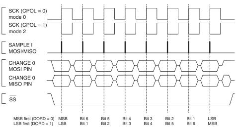
Figure 68. SPI Transfer Format with CPHA = 1
