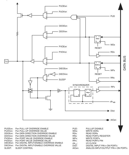
Note: 1. WPx, WDx, RRx, RPx, and RDx are common to all pins within the same port. clk<sub>I/O</sub>, SLEEP, and PUD are common to all ports. All other signals are unique for each pin.
