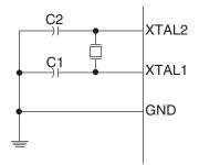
The Oscillator can operate in three different modes, each optimized for a specific frequency range. The operating mode is selected by the fuses CKSEL3..1 as shown in Table 4.
