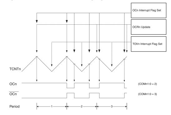
Figure 33. Phase Correct PWM Mode, Timing Diagram
