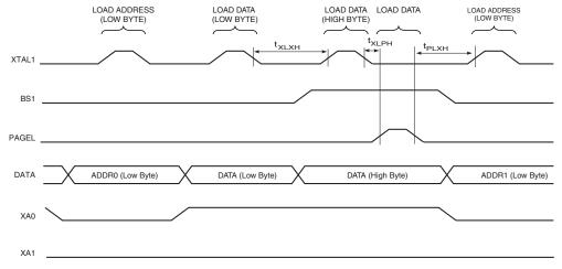
Note: 1. The timing requirements shown in Figure 133 (i.e., t<sub>DVXH</sub>, t<sub>XHXL</sub>, and t<sub>XLDX</sub>) also apply to loading operation.
