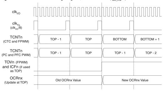
Figure 52. Timer/Counter Timing Diagram, with Prescaler ( $f_{clk}$  1/0/8)
