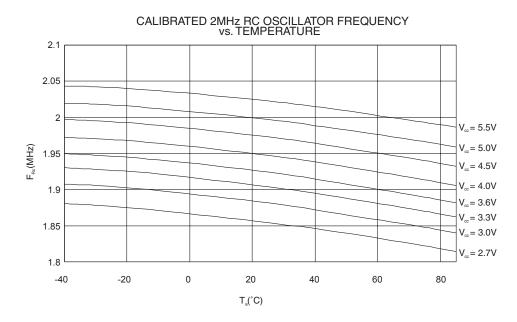
**Figure 150.** RC Oscillator Frequency vs. Temperature (the devices are calibrated to 2 MHz at Vcc = 5V, T=25c)
