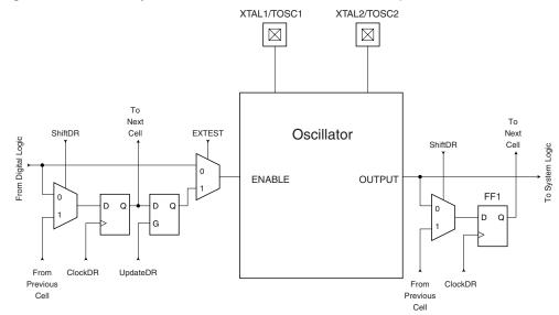
Figure 120. Boundary-scan Cells for Oscillators and Clock Options
