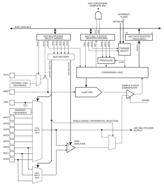
Figure 98. Analog to Digital Converter Block Schematic
