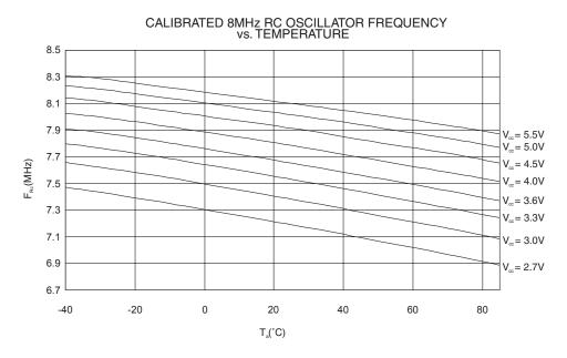
**Figure 155.** RC Oscillator Frequency vs. Operating Voltage (the devices are calibrated to 8 MHz at Vcc = 5V, T=25c)
