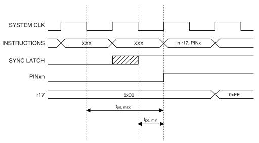
Consider the clock period starting shortly *after* the first falling edge of the system clock. The latch is closed when the clock is low, and goes transparent when the clock is high, as indicated by the shaded region of the "SYNC LATCH" signal. The signal value is latched when the system clock goes low. It is clocked into the PINxn Register at the
