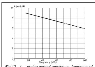
Fig.12. I<sub>Csat</sub> during normal running vs. frequency of operation for optimum performance
