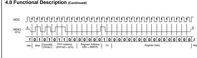
Figure 12. Typical MDC/MDIO Write Operation
