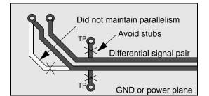
Figure 19. Differential signal pair
