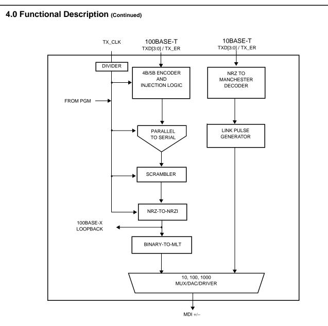
Figure 6. 10BASE-T/100BASE-TX Transmit Block Diagram
