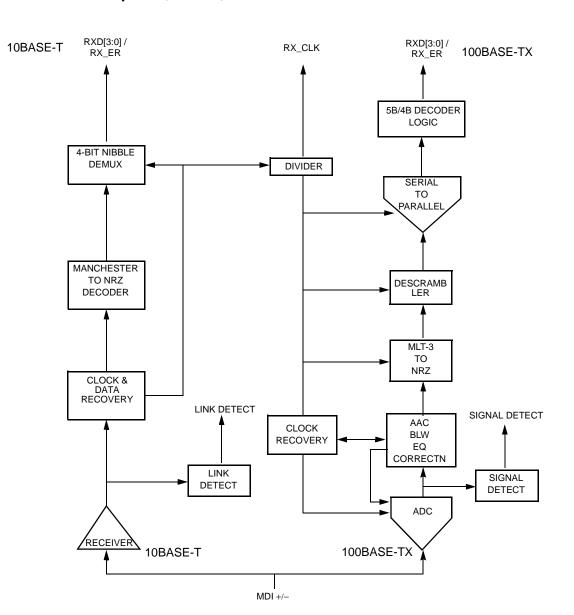
Figure 8. 10BASE-T/100BASE-T Receive Block Diagram
