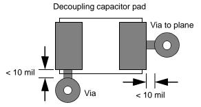
Figure 14. Place via close to pad.
