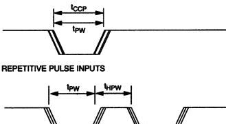
If during any pushbutton activity the STR input is activated, pushbutton operation will be suspended until the storage of EEPROM has been completed. Once complete, pushbutton inputs, if still active, will resume from the point of suspension. Command initiated storage operations will require a minimum of 4 ms to complete the storage operation. This 4 ms is measured from the rise of STR input (see Figure 5).
